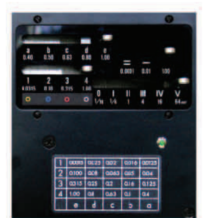
The diaphragms, the neutral density filter combination table and control levers
